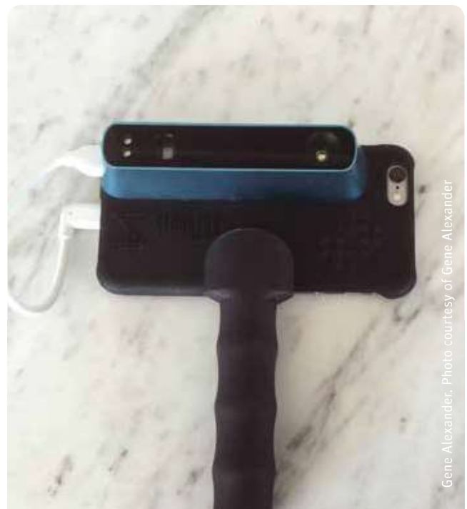
AutoAnthro, a new mobile device from Body Surface Translations (Athens, Georgia, US), derives child stature, head circumference, and mid-upper arm circumference from 3D scans and a 3D model.
